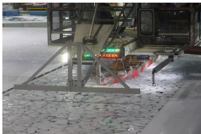
365 Figure 20: Ice model tests of 1:18.667 Araon hull model reported by Kim et al. [42]
