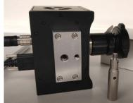
(a) Photonfocus camera setup with heat sinks
