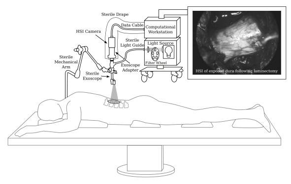
**Figure 1.** Schematic diagram of our intraoperative hyperspectral imaging (HSI) system illustrated for the example of spine surgery. A snapshot HSI camera system was used for the in-patient clinical feasibility case study as part of a spinal fusion surgery. Video-rate HSI data was acquired during surgery. An example *in vivo* snapshot hyperspectral mosaic image demonstrating the exposed dura of the spinal cord following laminectomy is provided.
