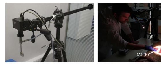
(a) iHSI camera system setup with tripod
