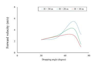
Figure 14: The lifeboat's after-launch forward speed at different dropping heights and angles.
