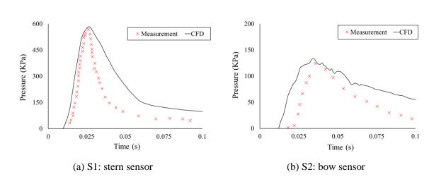
Figure 7: Comparison of time-series pressure between full-scale measurements and CFD using the Fine Mesh set (H = 30 m and  $\theta = 50^{\circ}$ ).
