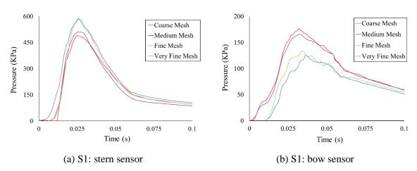
Figure 6: Time-series pressure predicted by CFD with different mesh densities (H = 30 m and  $\theta = 50^{\circ}$ ).
