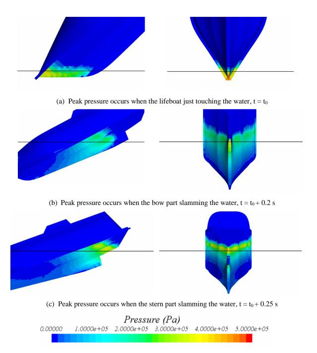
Figure 8: Water pressure impact on the lifeboat, presenting three moments when peak pressure impacts were observed (H = 30 m and  $\theta = 50^{\circ}$ ); left and right panels are respectively the profile and bottom view, and the undisturbed waterline is shown as a reference line.
