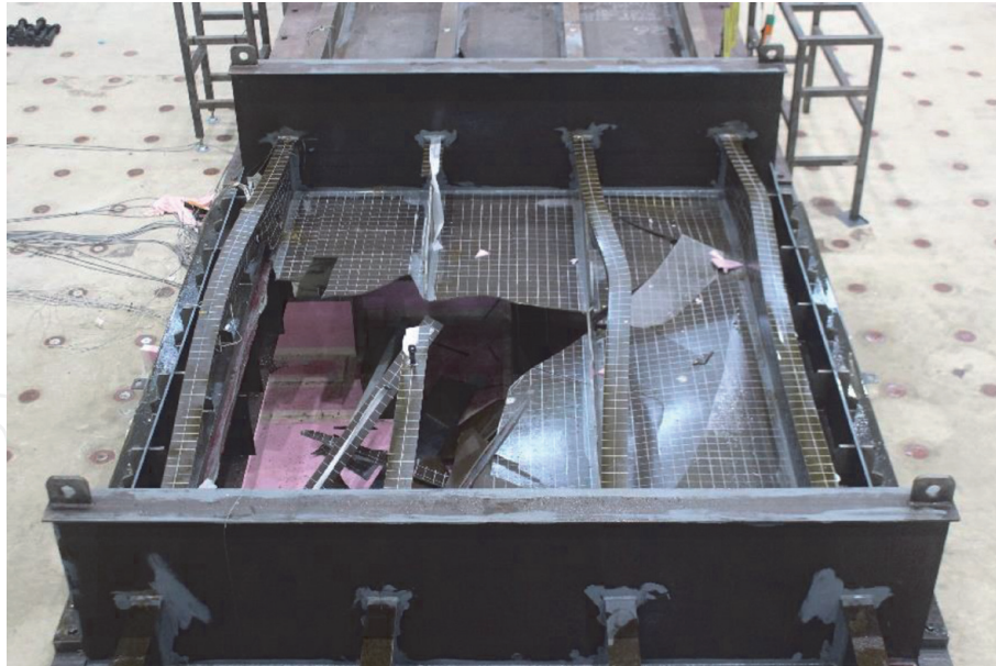
Figure 5. Brittle fracture of a full-scale steel stiffened plate structure under axial-compressive loads at -160^{\circ}\text{C} [7].
