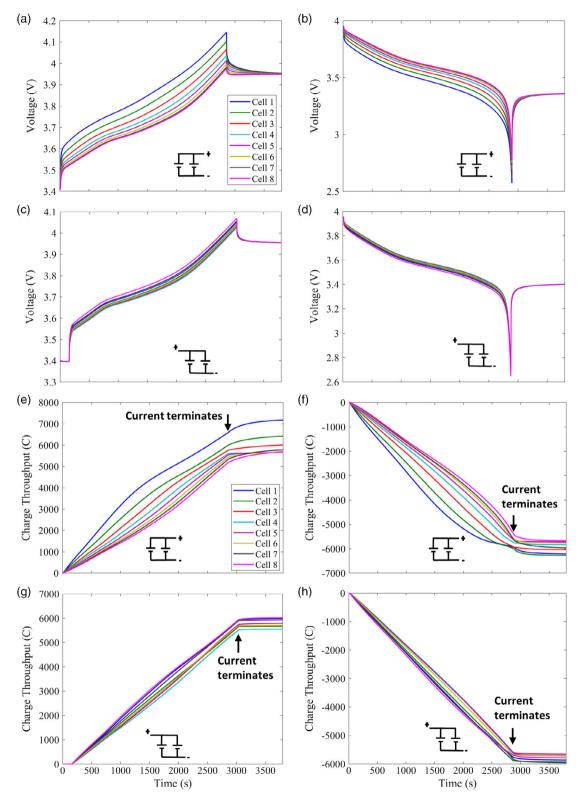
**Figure 5.** Voltage response of all cells during a,b) common-end operation and c,d) opposite-end operation. Cumulative charge for each cell during e) common-end charge, f) common-end discharge, g) opposite-end charge, and h) opposite-end discharge. The magnitude of the charge was used during the charge summation; therefore, the negative sign represents module discharge in (f) and (h).
