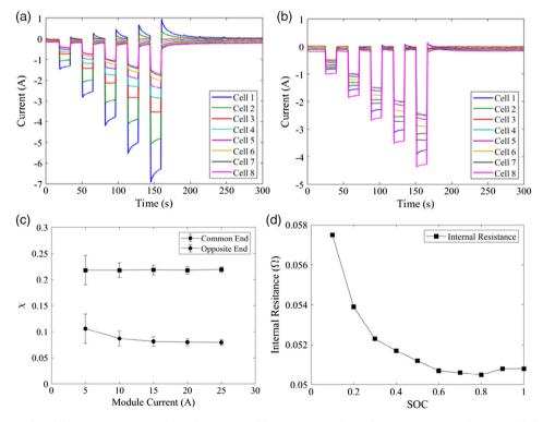
**Figure 6.** Cell currents of module in a) "common-end" configuration and b) "opposite-end" configuration. c) Ratio of current imbalance ( $\chi$ ) for different module currents and d) cell internal resistance at different SOCs. The internal resistance was obtained using galvanostatic EIS with the real resistance at 1 Hz taken for the plot.
