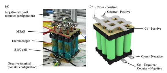
Figure 8. a) Image of the cell cluster and b) diagram showing different load electrical configurations.
