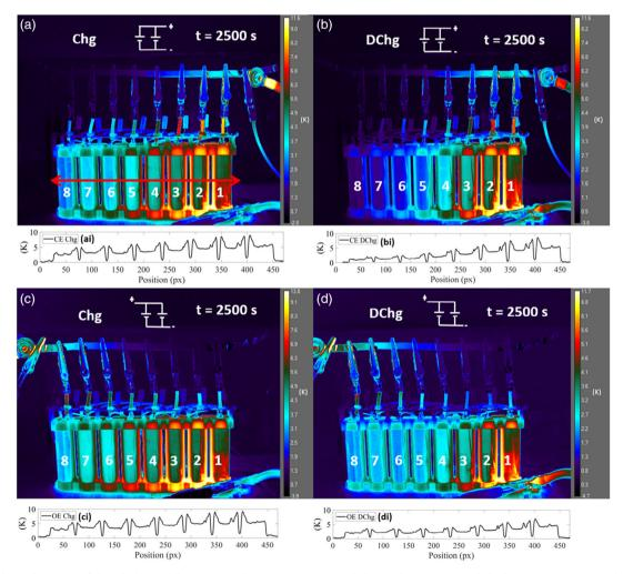
**Figure 7.** Thermal images of the whole module at 2500 s during a) common-end charge, b) common-end discharge, c) opposite-end charge, and d) opposite-end discharge. The numerical values in temperature scale represent temperature change.
