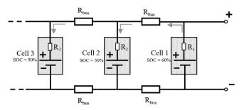
**Figure 1.** Parallel string of cells with different SOC levels. Example of cell rebalancing after charge. Cell 1 has a higher SOC due to the higher charge transferred from the lower resistive pathway to load. This results in rebalancing currents flowing from cell 1 into other cells in the parallel string.
