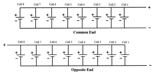
Figure 3. Electrical configuration of the module.
