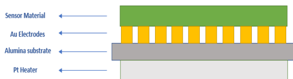
Fig. 1. Schematic of a NiO coated device in cross-section
