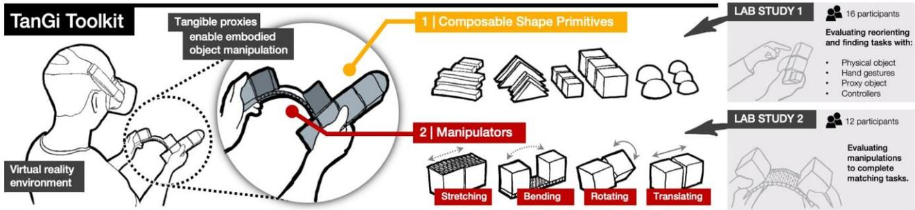
Figure 1: Visual abstract providing an overview of TanGi elements and the context of our two user studies. TanGi consists of *Composable Shape Primitives* allowing the approximation of a variety of objects, and *Manipulators* that provide movable proxy parts.
