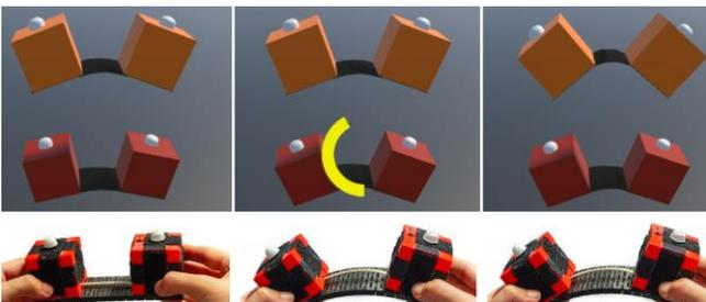
Figure 10: Study 2, the bending manipulator task: Each frame shows the required goal state (orange, top), the current registered state of the object (red, middle), and the corresponding proxy manipulation (bottom). Subjects were required to align both virtual objects, and maintain the position for two seconds; the center frame shows the progress indicator provided.
