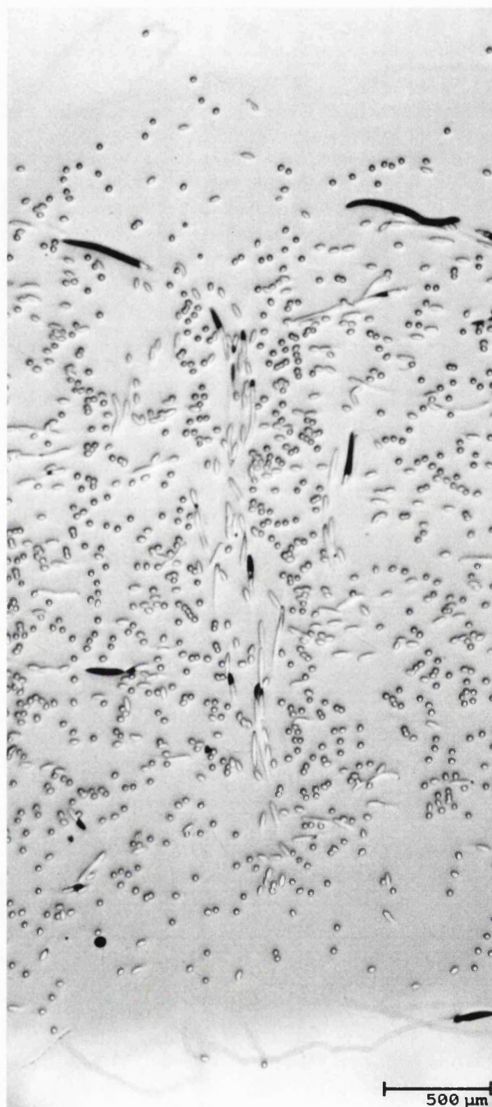
Figure 3.33: cross-section through the full thickness of the sample fabric (NP450P), showing a needle punch, or z-peg
