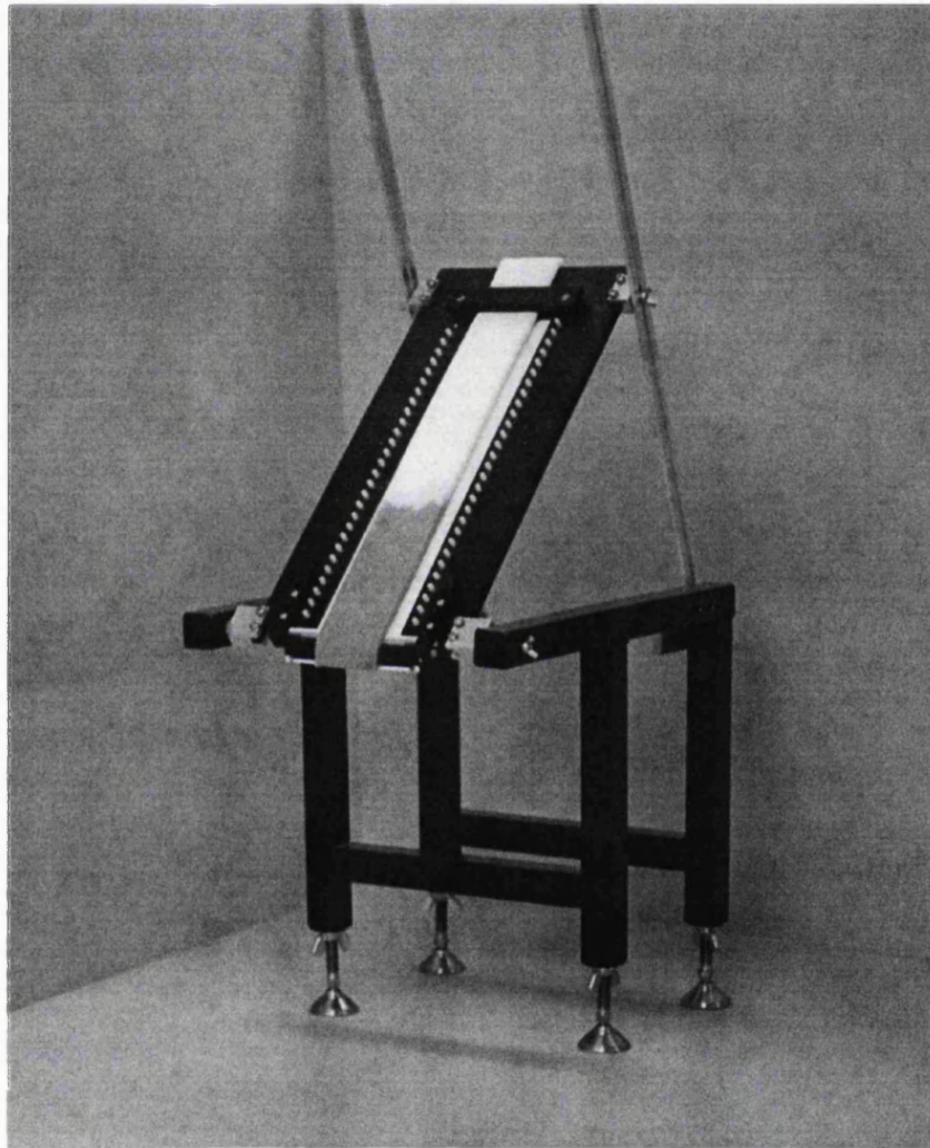
Figure 3.4: Photograph of apparatus to support a fabric sample horizontally, vertically, or at an intermediate angle (shown).
