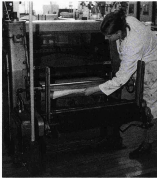
Figure 3.40: Needle loom, showing collection of needled fabric. (Texon UK Ltd pilot plant).
