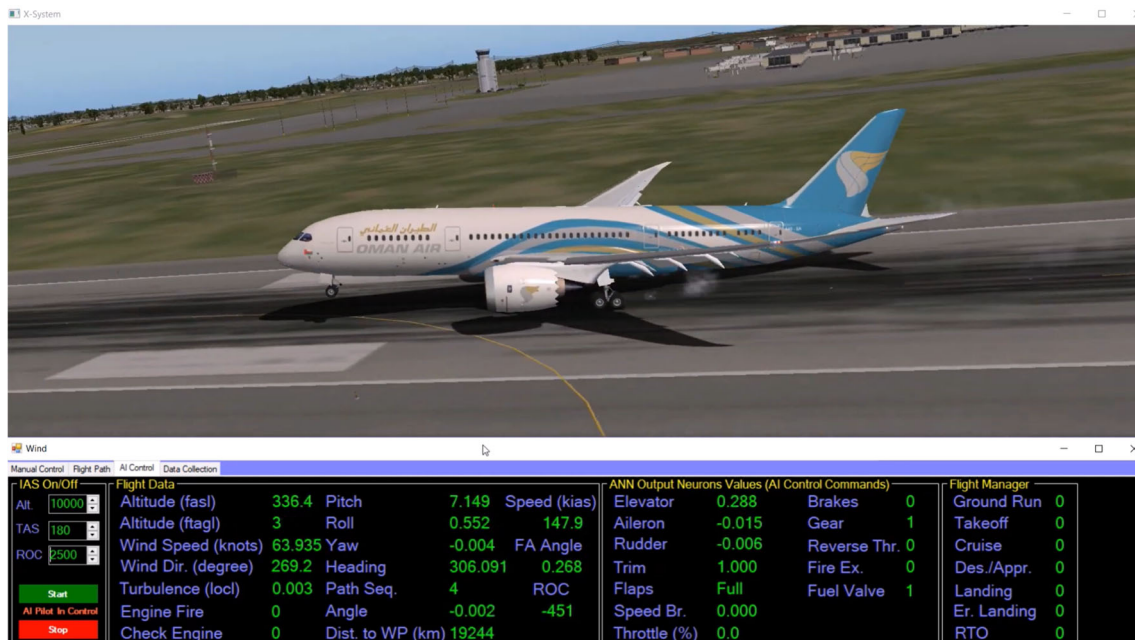
Fig. 33 The moment of touchdown on the landing runway by the IAS in the presence of extreme crosswind conditions beyond the current limits and capabilities
