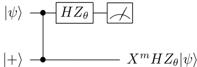
Figure 3.4: **Quantum circuit for teleporting a qubit rotated of an angle  $\theta$  around the Z axis.** Again, the initial state is an entangled state.  $HZ_\theta$  is applied to the first qubit. After measurement of the first qubit, the bottom line shows the final state of the second qubit.
