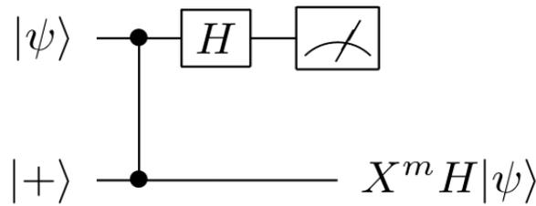
Figure 3.3: **Quantum circuit for teleporting a qubit.** The figure shows a pair of entangled states. A gate  $H$  is applied on the first qubit. The meter represents a measurement of which  $m$  is the outcome. The bottom line shows the final state of the second qubit.
