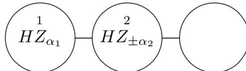
Figure 3.6: **Cluster state with three qubits.** Input prepared in the state  $|+\rangle$  and measurements of the form  $HZ_\alpha$  performed on the first two qubits.
