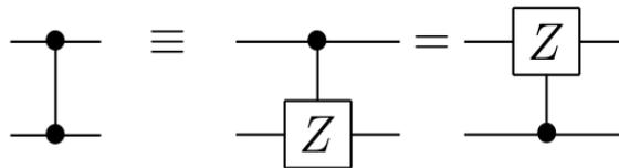
The controlled-phase acts as  $|x, y\rangle \rightarrow (-1)^{xy}|x, y\rangle$ .
