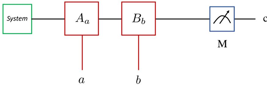
Figure 4.2: **Single-system protocol.** An initial system, which can be either a bit or a qubit, is subjected to controlled transformations, with control bits  $a$  and  $b$ , respectively, and then measured. The goal is to maximise the probability that the value of the output is the product of the values of the input bits.
