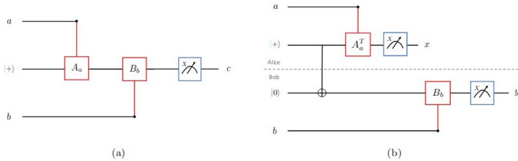
Figure 4.5: **Mapping of the CHSH\* game to the CHSH game.** Figure (a) shows the single qubit scheme, with the initial qubit in state  $|+\rangle$ , controlled gates  $A_a, B_b$ , measurement on the X basis and output  $c$ . Figure (b) shows the corresponding CHSH game, where Alice and Bob share a Bell pair, and apply gates  $A_a^T, B_b$  to their systems to obtain measurement results  $x$  and  $y$  respectively.
