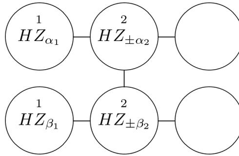
Figure 3.2: **A cluster-state computation [90]** The integers indicate the time ordering of the measurements. The qubits with associated single-qubit unitaries are the ones in which processing measurements occur. The remaining qubits are the output of the computation.
