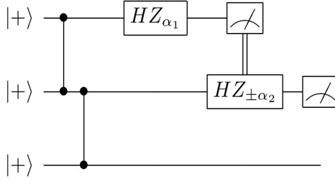
Figure 3.7: **Quantum circuit representation of the cluster state 3.6** The double vertical lines between the meter in the first qubit and the gate in the second qubit indicate the classical feed forward and control of later operations.
