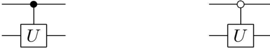
The top qubit is the control one and the bottom qubit is the target. In the circuit on the left,  $U$  acts on the target qubit if the control qubit is 1 and in the circuit on the right  $U$  acts on the target qubit if the control qubit is 0. One specific type of controlled-unitary gate that is often used is the controlled-not,
