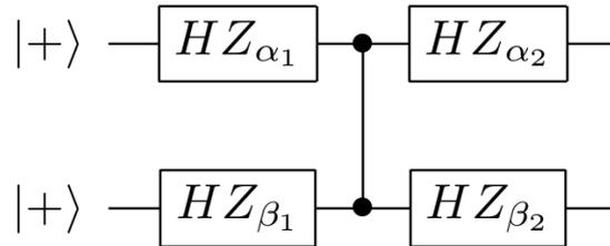
which can be simulated using the cluster state computation in 3.2. Conversely, any cluster state computation may be efficiently simulated in the quantum circuit model, and thus the two models are computationally equivalent. That way, just like the circuit model, the cluster-state model is also universal, which means that even though the results of the measurements in every step are random, any quantum computation can deterministically be realized.
