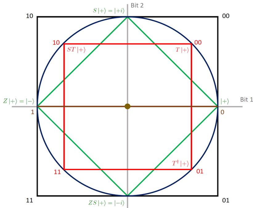
Figure 4.7: **Geometrical analysis of the protocol** The figure shows the state space of two bits (vertices of the big black square), one qubit ( $XY$  plane of the Bloch sphere) both in the optimal winning strategy (the vertices of the red square) and restricted to Clifford computation (the vertices of the tilted green square), and one bit, (e.g. the edges of the brown line). Notice that the measurement at the end of the protocol corresponds to the collapse of a state to the  $x$  axis.
