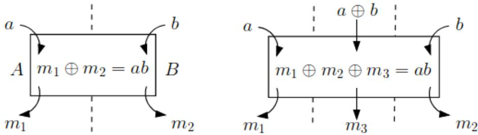
Figure 3.9: **AND as the parity of measurement outcomes.** The figure [3] shows an ideal nonlocal box defined to implement an AND and the measurements on a 3-qubit GHZ state implementing the same. The AND emerges as the parity of all outcomes. The NAND can be computed by a single NOT operation by the control computer.
