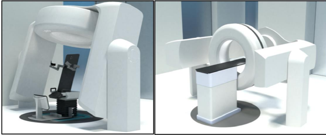
Figure 5.8: The MARIE DECT scanner shown with the EVE positioner for upright scanning and treatments and with a CT gurney for CT scanning in the lying down position.
