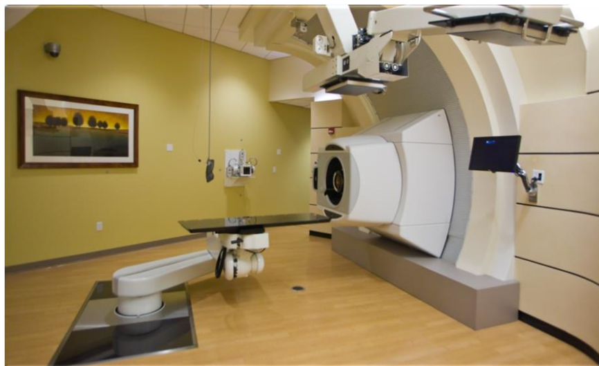
Figure 3.25. The Forte / Procure PPS as installed in one of the ProCure inclined beam treatment rooms at the Chicago center.
