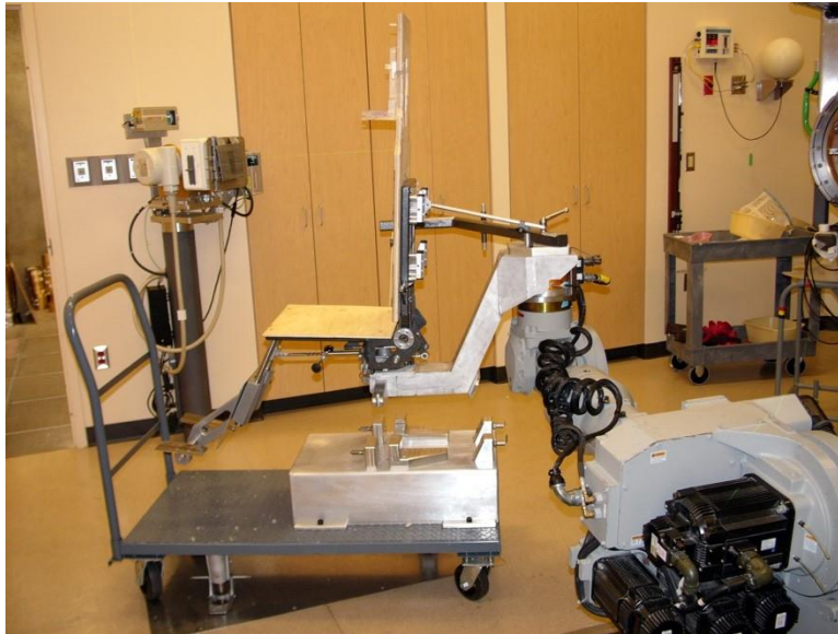
Figure 3.22. The treatment chair for intra cranial treatments in the fixed beam room. The transport cart secured in the docking position is also shown.
