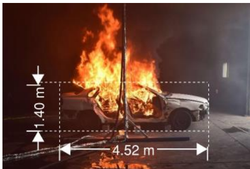
Figure 7 – Typical car fire test (prior to activation of the deluge system)
