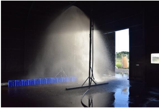
Figure 3 – Setup of the standard ‘pan tests’ for investigating water distribution from the nozzle. Blue square pans were positioned as shown in the photograph.
