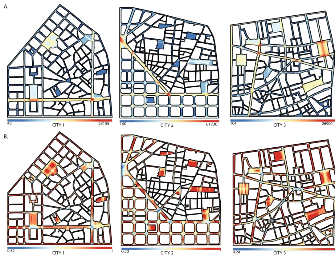
Figure 4. Visibility graph analysis (A) of the isovist area and (B) of the clustering coefficient.
