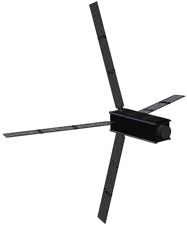
Figure 1: Geometry and configuration of the SOAR satellite with steerable fins and INMS payloads.
