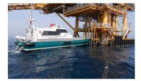
**Figure 3.** A crew boat snatching or mooring system to access an offshore platform
