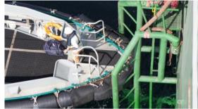
**Figure 4**. A crew boat snatching or mooring system to access an offshore platform
