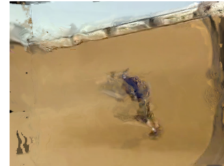
Figure 12: An output frame from the 'skateboarder' sequence where the system creates artefacts due to unreliable optical flow data between the seam frames.
