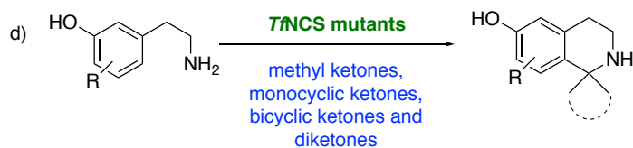
Scheme 1. Non-enzymatic and enzymatic routes to 1-monosubstituted and 1,1'-disubstituted PSRs. Parts (a) and (b) previous routes to 1,1'-disubstituted THIAs, (c) the use of imine reductases to enantiopure THIAs and (d) this work using NCS to 1,1'-disubstituted THIAs.
