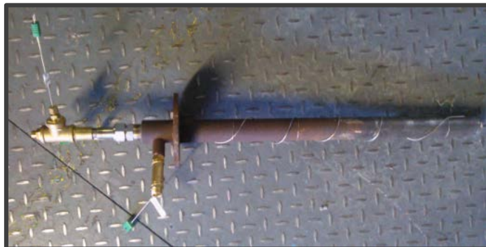
In-house air-cooled probe for convective heat flux measurement
