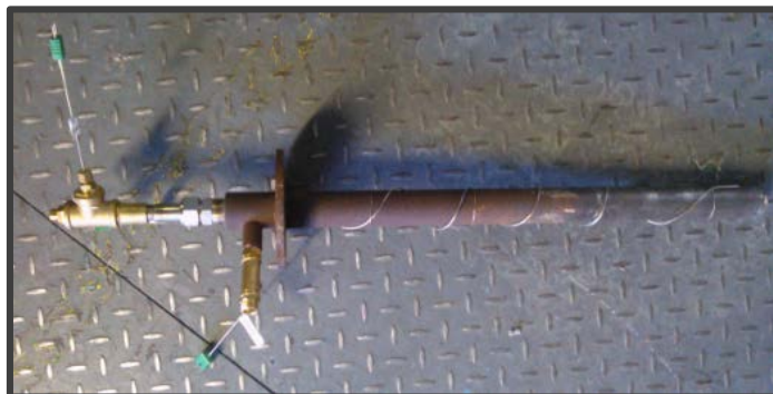
In-house air-cooled probe for convective heat flux measurement
