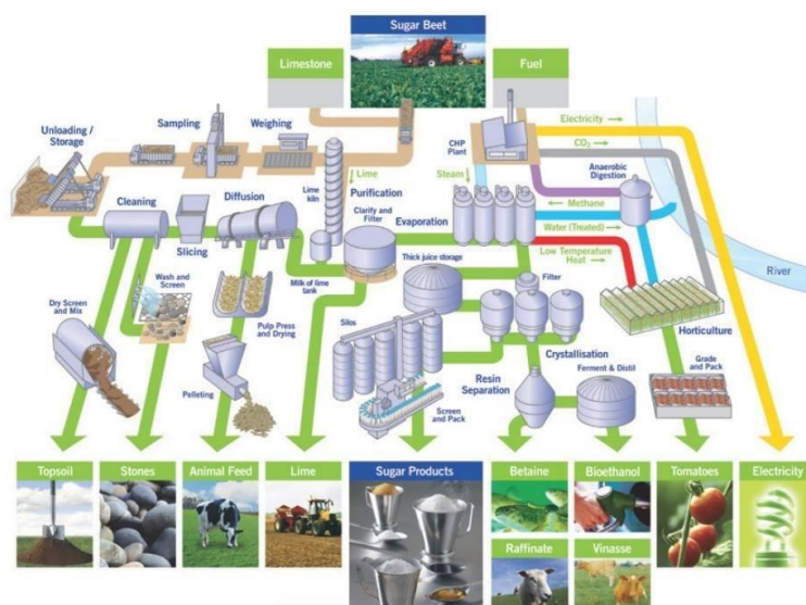
Figure 1.15. Schematic illustration of a biorefinery (Wissington, UK) for sugar beet processing to yield table sugar and a wide range of value-added co-products (British Sugar, 2011).
