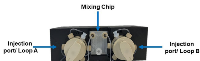
Fig. 7 Location of the mixing chip used for flow mixing experiments
