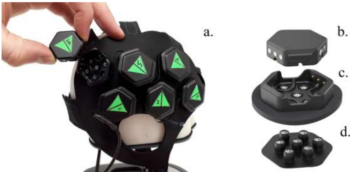
Figure 1. The cap containing 12 LUMO tiles in a 2 x 6 tile array, arranged to provide sensitivity to the superior temporal lobes and surrounding areas is shown in (a). Note the custom, adjustable neoprene cap that hosts the docks (c) into which the hexagonal tiles (b) are located. The light-guide piece shown in (d) contains seven short optical fibres with length 4.5 mm. Note the green high-contrast triangular labels, which supported photogrammetric registration.
