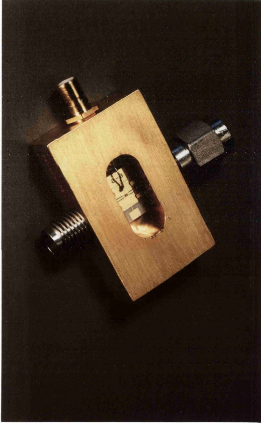
Figure 4.14. Photodiode mount with 6.6 mm long ceramic submount (photograph courtesy of Plessey Research Caswell)
