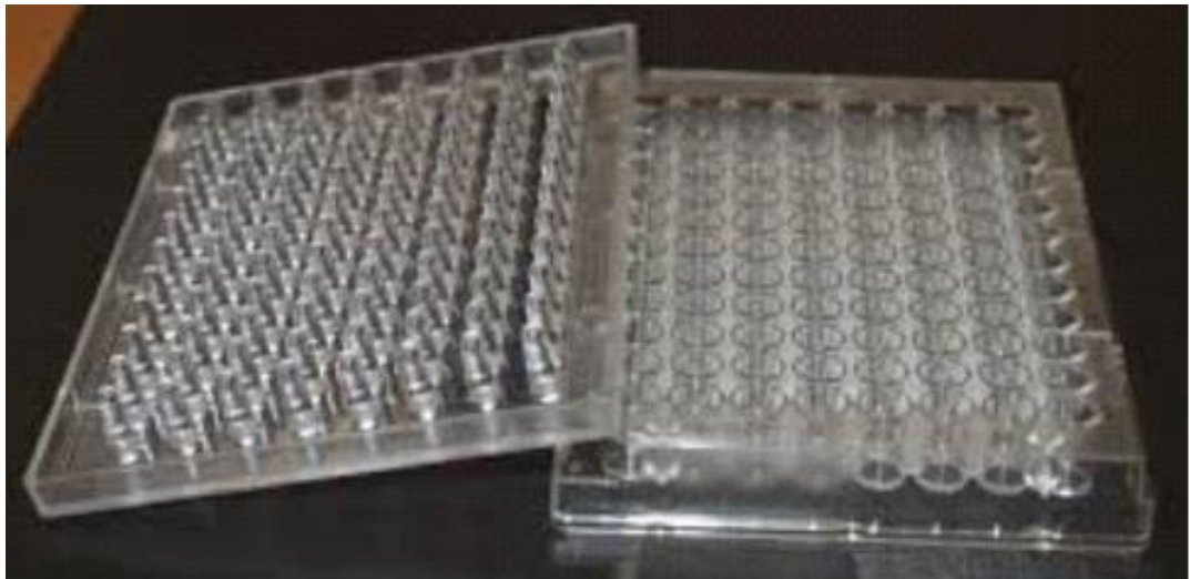
Figure 53 - Calgary biofilm device – Lid with pegs, where biofilm grows, and the base, a 96 well plate.
