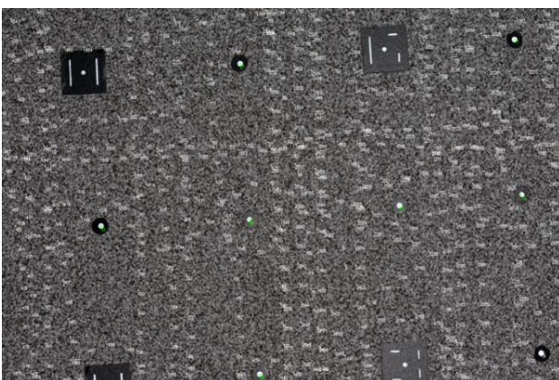
Figure 8. T-probe measurement locations back-projected onto image using photogrammetric lens model.
