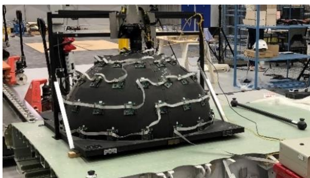
Figure 1. The 0.5m radius UCL illumination dome. Coded targets to characterise and track the dome are visible at the corners of the dome base plate and on the dome surface.
