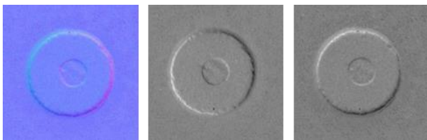
Figure 12. Detail 300x300 pixels of retro target in (left) normals; (centre) X gradients; (right) Y gradients.
