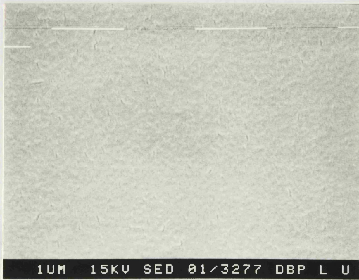
FIGURE 60 Scanning electron micrograph showing the surface structure of the lower surface of the film described in Figure 59. Magnification x 13800: Sample Tilt Correction 30°.
