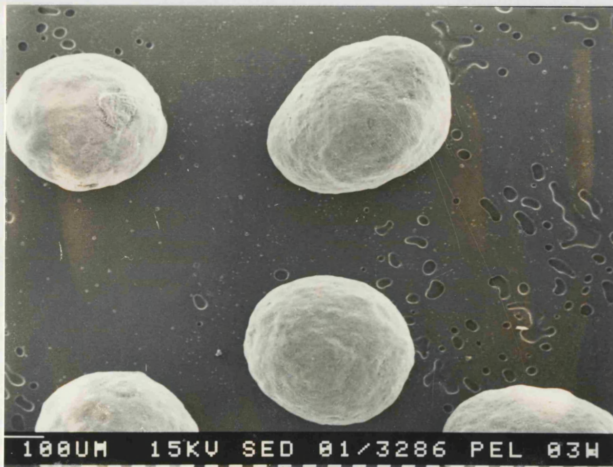
FIGURE 119 Scanning electron micrograph showing the surface structure of a non-pareil pellet coated with a film containing equal proportions of Eudragit RL and Eudragit RS with 10% w/w glyceryl triacetate and 5% w/w oxamniquine (relative to total polymer weight). (FORMULATION A1). Magnification x 14: Sample Tilt Correction 0°.
