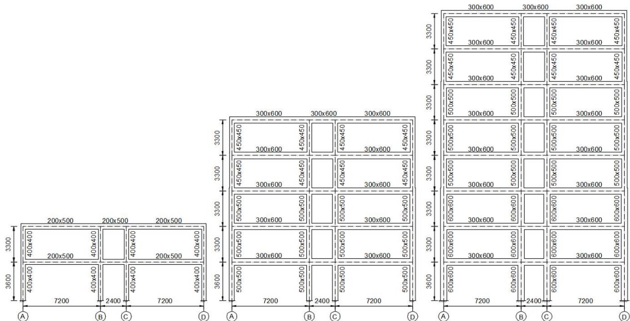
Fig. 8 - Structural member sections for (a) 2-storey, (b) 5-storey and (c) 8-storey index buildings.
