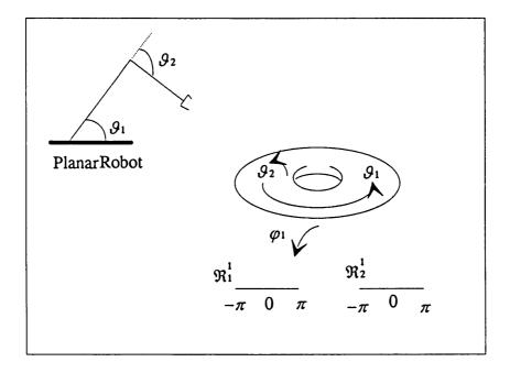
Figure 4-6: Joint Space Manifold for a 2R Planar Robot
