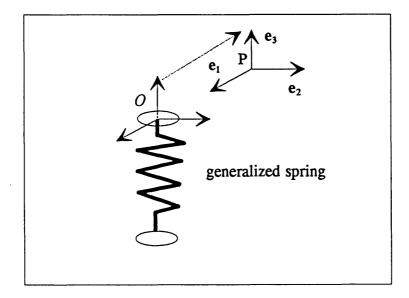
Figure 7-3: Generalized Spring with Shifted Reference Frame
