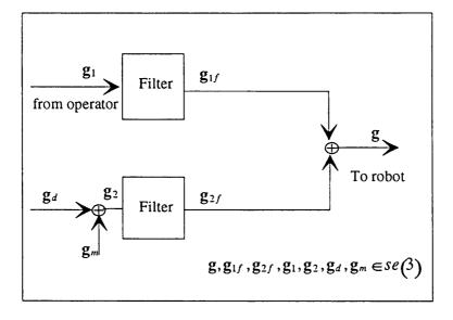
Figure 6-2: Conceptual Design for Simple Shared Controller
