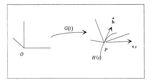
Figure 4-3: Moving Reference Frame
