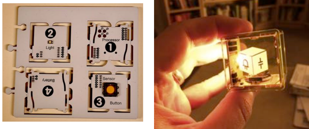
Figure 6.4: (left) The MakeMe printed circuit board before being assembled, (right) the assembled MakeMe cube with a glowing neopixel light.
