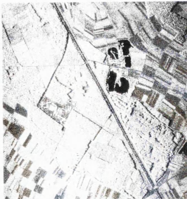
Fig.1.3 SAR 580 images, HH polarisation, forested areas and agricultural fields, A. L band B. X band (after M.G. Wooding, 1988)
