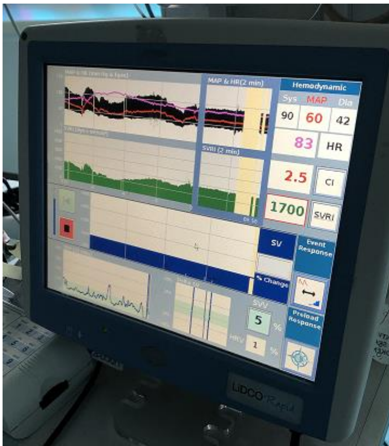
Figure 5.1: The LiDCOrapid Pulse Contour Analyser. The pulse contour analyser is plugged into the monitor module which received input from the arterial transducer. Data that generates the arterial waveform are analysed by the pulse contour analyser to provide estimates of haemodynamic variables. The blood pressure (systolic, mean and diastolic), heart rate (HR), cardiac index (CI) and systemic vascular resistance index (SVRI) measurements are displayed in real time.
