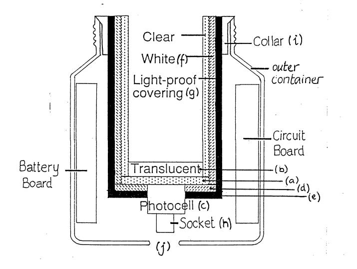
Figure 4.3 Diagrammatic Representation of a Cross Section of the Device. For an explanation of the letters see text.
