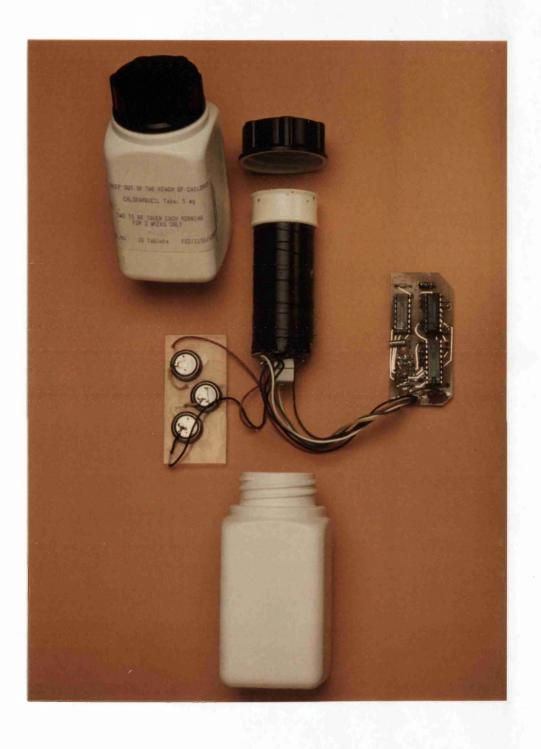
Figure 4.1 Photograph of the Electronic Recording Device and its Component Parts
