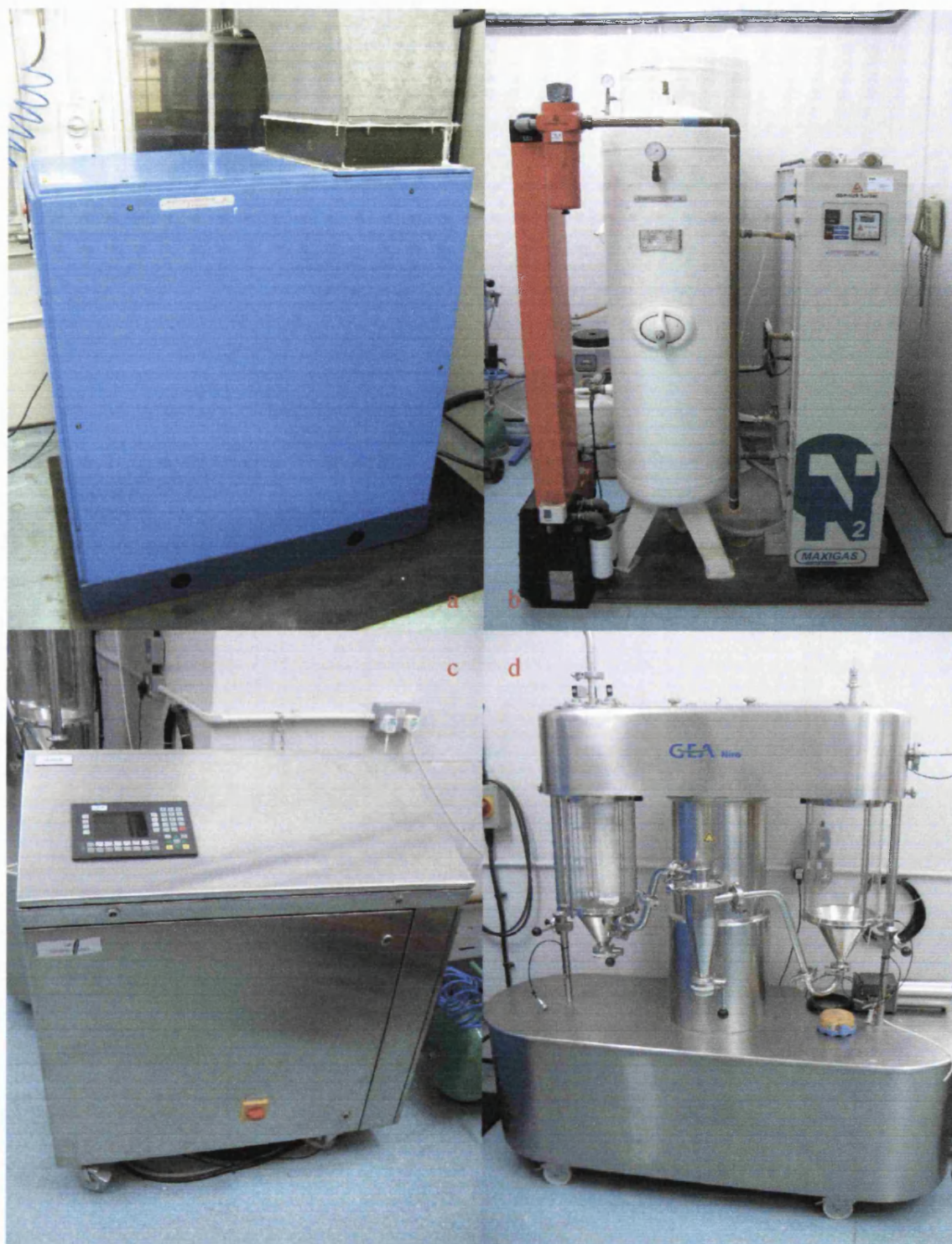
Figure 2.9: A picture of the Niro SD MICRO TM spray drying unit which includes a) air compressor, b) nitrogen generator, c) operating control panel and d) spray dryer.
