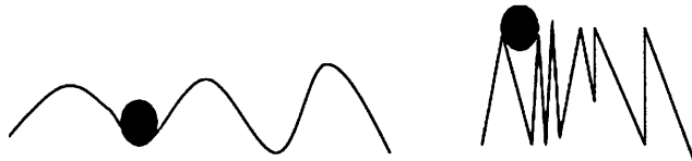
Figure 5.8. Left is a schematic image of a smoother surface with longer peak-to-peak distance, right is a rougher surface with shorter peak to peak distance and left the smoother surface with longer peak-to-peak distance.
