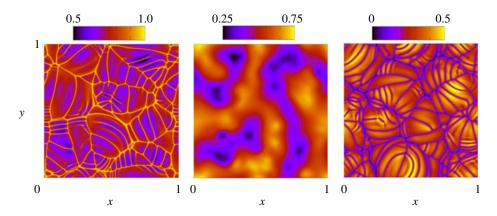
**Figure 4.** Slices of the temperature field in a three-dimensional 'two-sided' cell, at depths, from left to right, z = 30/Ra (near the lower boundary), z = 0.5 (the midplane), and z = 1 - 30/Ra (near the upper boundary), for Ra = 8000. Taken from [58]. (Online version in colour.)
