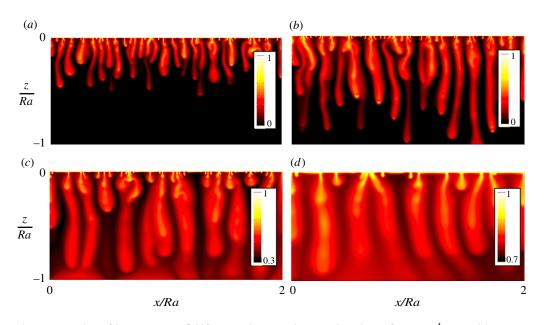
**Figure 7.** Snapshots of the concentration field from two-dimensional numerical simulations for  $Ra = 10^4$  at times (*a*) t = 4Ra, (*b*) t = 8Ra, roughly when the plumes first hit the base, (*c*) t = 32Ra and (*d*) t = 128Ra. Note the changing colour scale as the domain fills up with solute. Adapted from [40]. (Online version in colour.)
