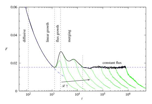
**Figure 8.** The buoyancy flux *F* through the upper boundary from simulations in a two-dimensional medium for a series of different values of *Ra* between *Ra* = 100 and *Ra* =  $5 \times 10^4$ , taken from Slim [36]. The behaviour of the flux changes as the flow evolves through the different dynamical regimes marked. The only effect of the lower boundary—that is, *Ra*—is to determine the time at which the flow enters the final, 'shutdown' regime. (Online version in colour.)
