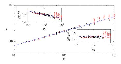
**Figure 5.** The dominant horizontal wavenumber of the interior flow for two-dimensional porous convection, taken from [38] (black stars) and [34] (red circles), together with the fit  $k = 0.48Ra^{0.4}$  (blue line). The insets shows the same data scaled by  $Ra^{0.5}$  and  $Ra^{0.4}$  as marked. (Online version in colour.)
