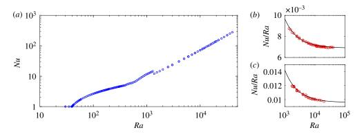
**Figure 2.** (*a*) The dimensionless flux *Nu* as a function of *Ra* from numerical simulations of two-dimensional 'two-sided' convection, taken from [38]. (*b*) The scaled *Nu* in the high-*Ra* regime, together with the fit (3.6) (solid line). (*c*) The scaled *Nu* in the high-*Ra* regime from equivalent three-dimensional simulations (taken from [58]), together with the fit referenced in the text (solid line). (Online version in colour.)
