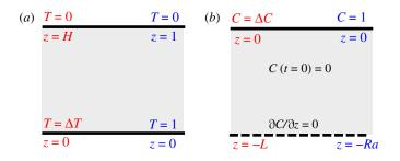
**Figure 1.** Simple schematics of (*a*) the 'two-sided' and (*b*) the 'one-sided' systems, shown in two dimensions with dimensional labels (red, left) and equivalent dimensionless labels (blue, right) according to the scalings discussed in the main text in each case. (Online version in colour.)
