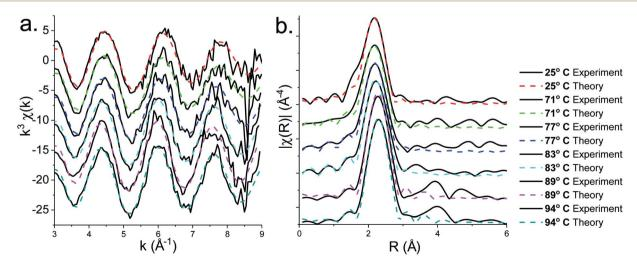
(a) EXAFS and (b) FT fits for the solvothermal decomposition of 1 in oleylamine at 25 °C, 71 °C, 77 °C, 83 °C, 89 °C and 94 °C.
