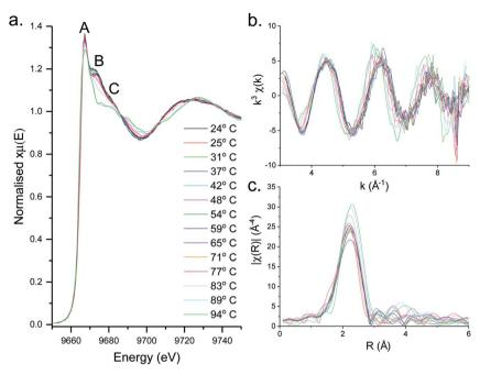
Fig. 5 In situ (a) XANES spectra, (b) EXAFS and (c) FT of the solvothermal decomposition of 1 in oleylamine up to 94 °C at a ramp rate of 1 °C min<sup>-1</sup>. The relevance of the peaks marked (A-C) is discussed in the text.
