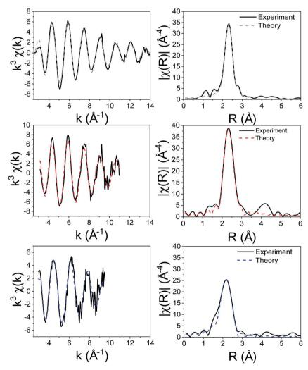
Fig. 4 k<sup>3</sup>-Weighted EXAFS and Fourier transformed (real space) data of 1 solid (top), in xylene (middle) and in oleylamine (bottom).
