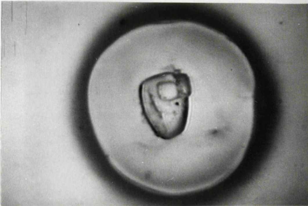
Figure 7.14a Photograph of sodium chloride starting to recrystallise under B72 film after removal from high RH. Photograph taken from the video.
