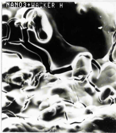
Figure 7.2 SEM SEM photograph of sodium nitrate and Wacker H. Cracks in the polymer film can be seen.
