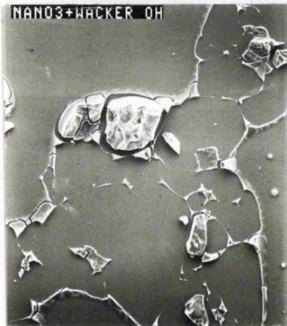
Figure 7.3 SEM SEM photograph of sodium nitrate and Wacker OH. Salts have become detached from the surface of the slide despite consolidation. In areas where no salts were originally present (top left and bottom right), a flawless film has formed.
