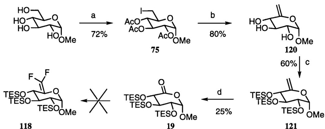
Conditions: a) i.  $\text{Ph}_3\text{P}$ ,  $\text{I}_2$ , imidazole, toluene,  $70^\circ\text{C}$ ; ii.  $\text{Ac}_2\text{O}$ , pyridine, r.t.; b) i. DBU, THF, reflux; ii.  $\text{NaOMe}$ ,  $\text{MeOH}$ , r.t.; c)  $\text{Et}_3\text{SiCl}$ ,  $\text{Et}_3\text{N}$ ,  $\text{NaH}$ , DMAP, DCM, reflux; d) i.  $\text{O}_3$ , DCM,  $-78^\circ\text{C}$ ; ii.  $\text{Me}_2\text{S}$ .
