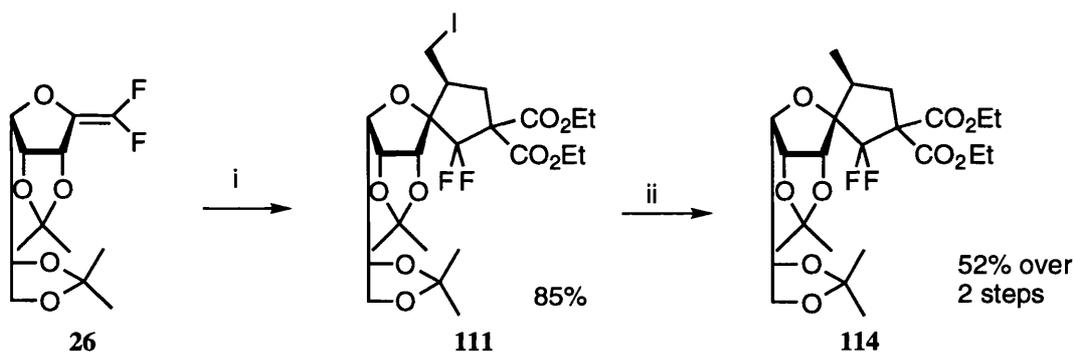
Conditions: i. **109**,  $\text{Bu}_3\text{SnSnBu}_3$ ,  $\text{hv}$ , benzene, r.t.; ii. AIBN,  $\text{Bu}_3\text{SnH}$ , benzene, reflux.
