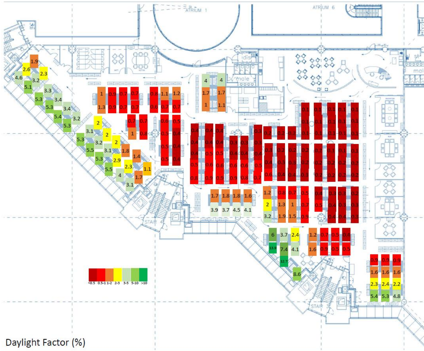
Figure 6- 3: Point daylight factor calculated at the centre of each desk (plane height: 0.8m)
