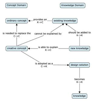
Fig. 2 A schematic illustration of C-K theory operators (Sharif Ullah et al, 2012)
