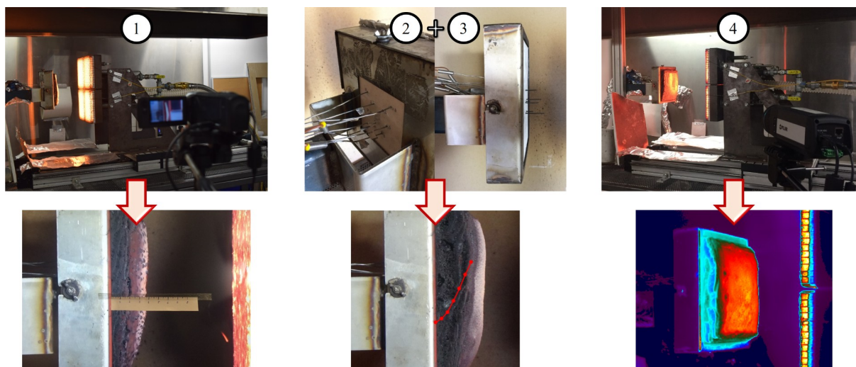
Fig. 2. Different aspects of the experimental setup designed to gauge the thermo-physical response of intumescent coatings during heating exposure.
