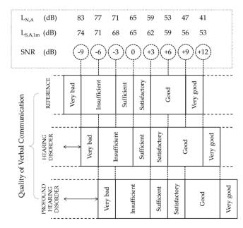
**Figure 4.** Threshold values of speech levels and ambient noise levels for the quality of verbal communication and its relation to SNR as suggested: by Lazarus [38] for reference listeners; inferred from ISO 9921 for listeners with slight hearing disorders [39]; hypothesised for listeners with profound hearing disorders [40].
