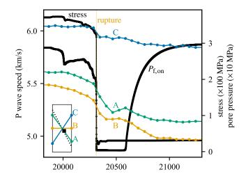
Figure 3: Test conducted at  $P_c = 70$  MPa and  $P_f = 30$  MPa. Evolution of differential stress, on-fault pore pressure, and P wave speed along (path A, green) and across (paths B, orange, and C, blue) the fault during rupture.
