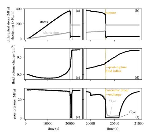
Figure 2: Test conducted at  $P_c = 70$  MPa and  $P_f = 30$  MPa. Differential stress and axial shortening (a,b), fluid volume change (c,d) and on- and off-fault pore pressure (e,f) as a function of time during the triaxial rupture experiment. Panels (b,d,f) correspond to the time period marked between the thin vertical lines in panels (a,c,e).
