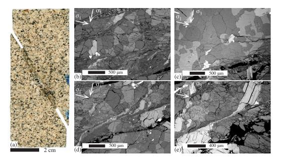
Figure 7: Fault zone structure in the sample tested at  $P_c = 70$  MPa and  $P_f = 30$  MPa. (a) Optical image of the whole sample after polishing (notches were filled with a Teflon sheet during the test itself). (b–e) SEM Backscattered electron images of the internal structure of the fault; the orientation of remotely applied principal stresses is indicated by the white arrows.
