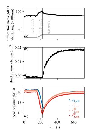
Figure 5: Test conducted at  $P_{\rm c} = 60$  MPa and  $P_{\rm f} = 20$  MPa. See Figure S1 for sample geometry and labelling of pore pressure transducers. Differential stress and axial shortening (a), fluid volume change (b) and on- (red) and off-fault (blue) pore pressure (c) as a function of time during a slip-rate step from 1.15 to 11.5  $\mu$ m/s.
