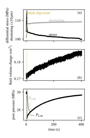
Figure 4: Test conducted at  $P_c = 70$  MPa and  $P_f = 30$  MPa. Differential stress and axial shortening (a), fluid volume change (b) and on- and off-fault pore pressure (c) as a function of time during a stick-slip event.
