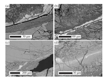
Figure 8: Fault zone structure in the sample tested at  $P_{\rm c} = 70$  MPa and  $P_{\rm f} = 30$  MPa. (a–d) SEM Backscattered electron images of the thin shear zones occurring within the fault gouge layer. In image (c), the large black region is an area where the gouge material was lost during sample preparation.
