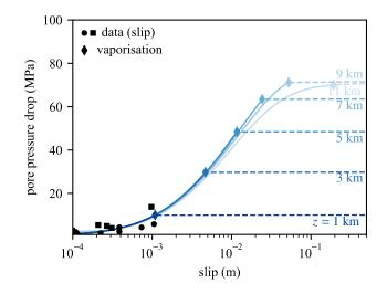
Figure 9: Isothermal, undrained pore pressure drop as a function of slip for a range of depths. Black circles and squares show laboratory data obtained during slip in the tests conducted at  $(P_c, P_f) = (70, 30)$  and  $(P_c, P_f) =$ (60, 20), respectively. Diamonds indicate points where fluid vaporisation occurs. An initial porosity of 2% was used. At each depth, the initial pore pressure is assumed hydrostatic, and the initial temperature is computed using a 40°C km<sup>-1</sup> geotherm.
