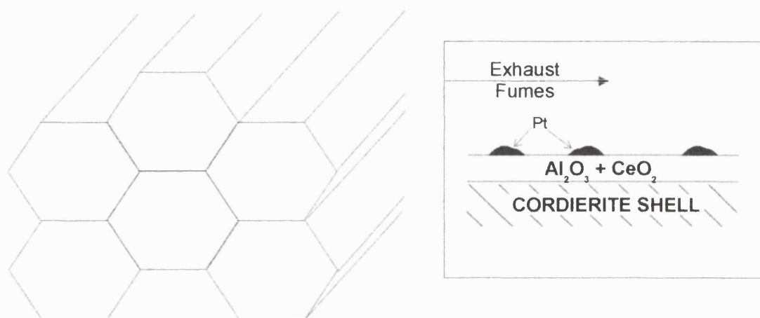
Figure 3.1: Schematic of an Automobile Exhaust Three-Way Catalytic Converter, illustrating the honeycomb cordierite shell of the device, and a closer view of the surface of the shell.
