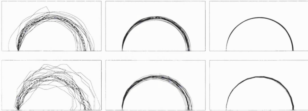
Figure 5.5: example tracks ( n = 20 ) computed using model A to illustrate the effects of noise and interpolation. Top row: using tri-linear interpolation; Bottom row: using nearest-neighbour interpolation. Left: \text{SNR} = 8 ; middle: \text{SNR} = 32 ; right: \text{SNR} = 128 . The ideal track is shown by a dotted line (visible in the left hand images). All plots were produced with a fractional anisotropy of 0.4 and a radius of curvature of 4 pixels, using a step size of 0.02 pixels.
