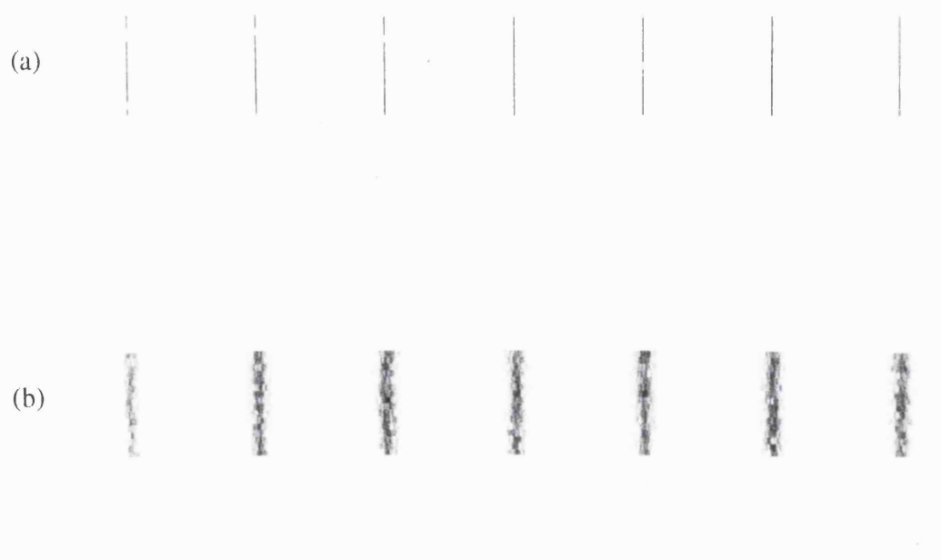
Figure 4.1 Geometric image from (a) hypothetical situation where no spread occurs and (b) conventional lead collimator.
