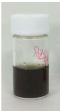
Figure 3-28 Picture of Fe NPs transferred in water using PIMA-Dopa polymer.
