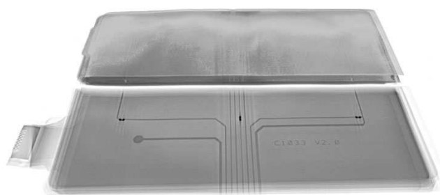
Figure 2. Instrumented cell reconstructed X-ray CT image. Half of the sensor assembly is shown, fitting accurately in the middle of the electrode stack. No damage to the electrodes or the sensor was observed.
