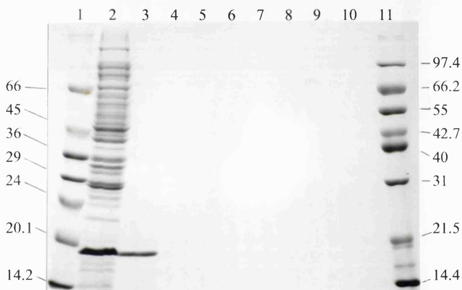
Figure 5.12 Photograph of a 15% Coomassie-stained SDS-PAGE gel with concentrated samples from the Elute 1 fractions of the beads charged with selected metal ions (in 0.1 M sodium acetate, 0.5 M NaCl, pH 3.8) and loaded with clarified extract - see section 5.13.1. Lane 1 , 5 \mu l molecular weight markers (Sigma, SDS-7); lane 2 , 161 \mu l, loaded clarified extract; lane 3 , 82.5 \mu l tube 1 ( \text{CuCl}_2 ); lane 4 , 82.5 \mu l tube 2 ( \text{ZnCl}_2 ); lane 5 , 82.5 \mu l tube 3 ( \text{NiCl}_2 \cdot 6\text{H}_2\text{O} ); lane 6 , 82.5 \mu l tube 4 ( \text{MgCl}_2 \cdot 6\text{H}_2\text{O} ); lane 7 , 82.5 \mu l, tube 5 ( \text{CaCl}_2 \cdot 2\text{H}_2\text{O} ); lane 8 , 82.5 \mu l tube 6 ( \text{FeCl}_2 \cdot 4\text{H}_2\text{O} ); lane 9 , 82.5 \mu l tube 7 ( \text{FeCl}_3 \cdot 6\text{H}_2\text{O} ); lane 10 , 82.5 \mu l tube 8 (uncharged/IDA); lane 11 , 5 \mu l molecular weight markers (Promega, Mid-Range). The sizes of the molecular weight markers are in kDa.
