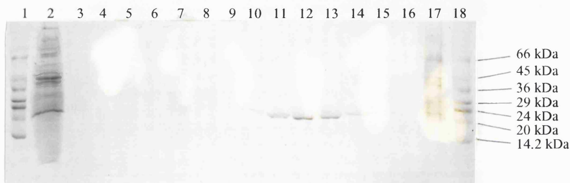
Figure 4.6 Photograph of a 12% SDS-PAGE gel loaded with samples from a HiTrap column charged with Cu showing the purification of the recombinant T4 lysozyme - column 3. The samples in lanes 2-17 inclusive were concentrated 10-fold with TCA precipitation and 20 \mu l were loaded into the wells. Lanes 1 and 18 , 5 \mu l molecular weight markers (Sigma, SDS-7); lane 2 , 20 \mu l of the extract loaded onto the column ; lane 3 , fraction 5; lane 4 , fraction 10; lane 5 , fraction 20; lane 6 , fraction 25; lane 7 , fraction 30; lane 8 , fraction 32; lane 9 , fraction 34; lane 10 , fraction 36; lane 11 , fraction 38; lane 12 , fraction 40; lane 13 , fraction 42; lane 14 , fraction 44; lane 15 , fraction 46; lane 16 , fraction 48; lane 17 , fraction 51.
