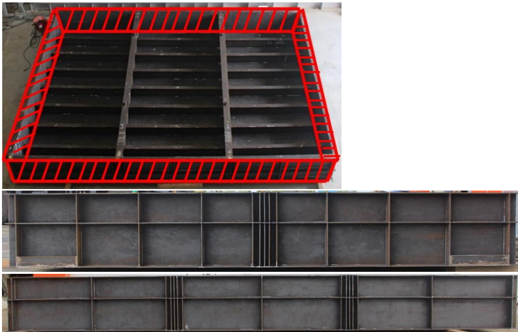
Figure 10. Fabrication of support jigs along four boundaries of the test structure.
