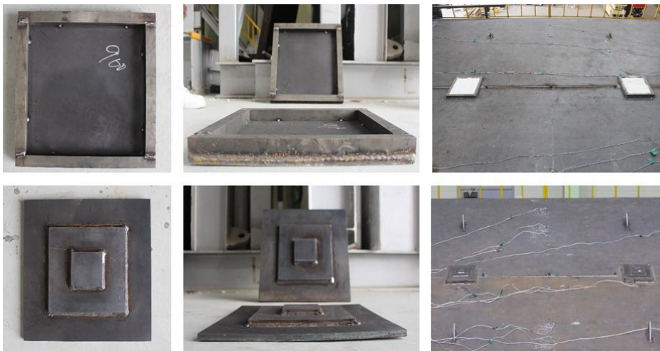
Figure 20. Manufactured and installed patch load plates.
