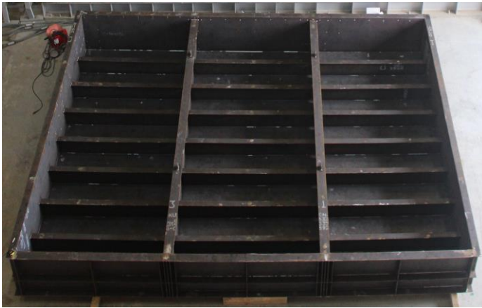
Figure 9. The fabrication process at the shipyard: (a) raw plate sheet, (b) plate cutting, (c) assembly of support members and support jigs, (d) completion of the test structure.
