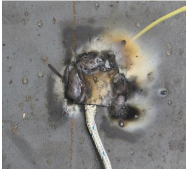
Figure 25. Spot welding to attach thermo-electric couple sensors.
