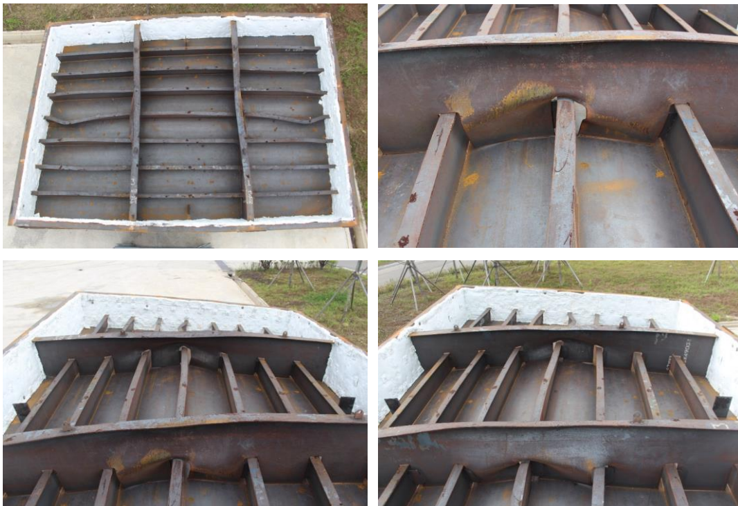
Figure 35. Deformed shapes of the test structure after the test.
