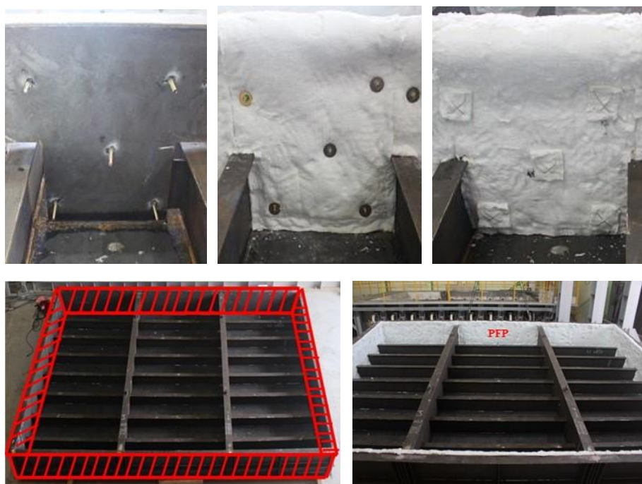
Figure 16. Insulation with passive fire protection material along the four boundaries of the test structure.
