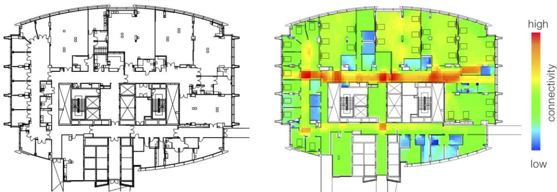
Figure 4. (left) A floor plan used to model a visibility graph on eye-level using only solid walls as barriers; (right) visualisation of the measure of connectivity, showing highly connected spaces as warm colours and spaces with low connectivity as cool colours
